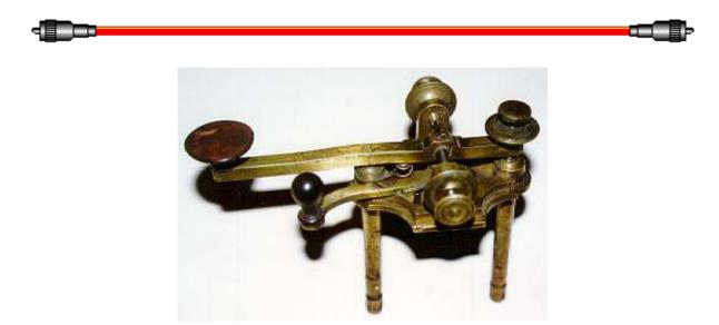
This early straight lever key was made by the Caton Instrument Co., Ottawa, Ill. The long legs pass through holes in the operating table and wires are attached to binding posts at the end of each leg. Circa 1860's
