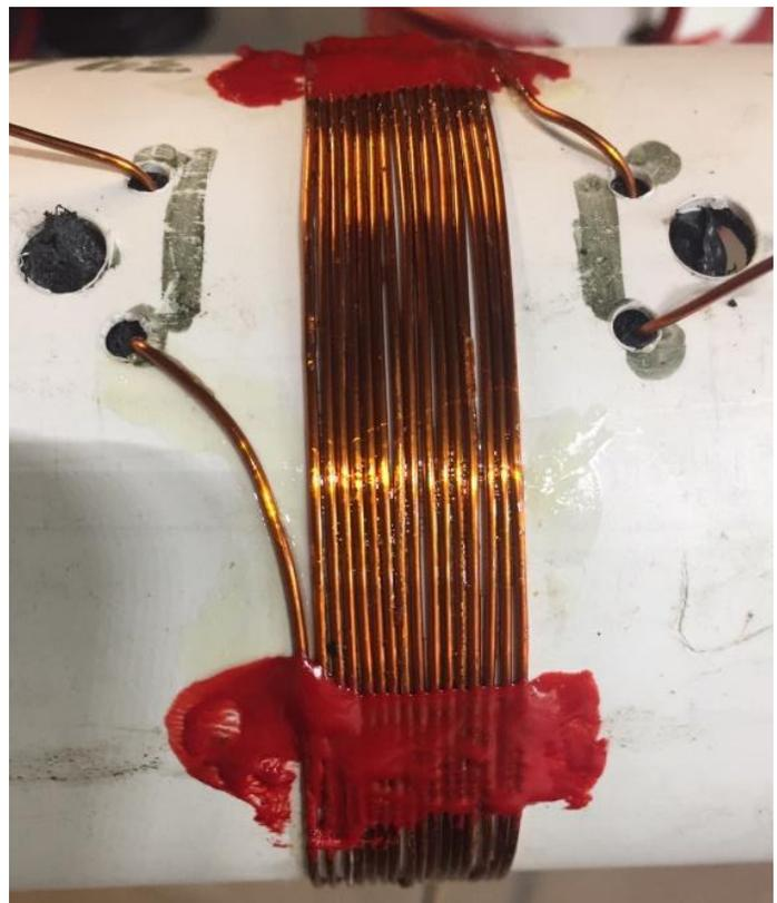
Once wound and measured, the coil is coated in 5 places with liquid electrical tape to hold it in place. It causes no change in L.
