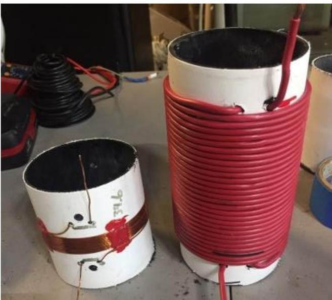
Above -- One using #20 enameled and the other using #10 insulated. Both produced a 35 uH coil, but the red coil was significantly heavier and would cause MAJOR antenna drooping.
