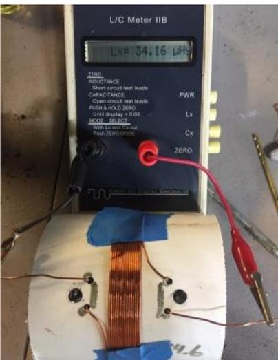
Left shows the measurement of the #20 coil with the AADE L meter.
