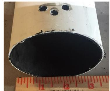
The 3.3" PVC is cut to a needed length which is, typically, coil width plus 1 inch on either side for support insulator fastening. The above was my long form for the #10 insulated wire coil.
