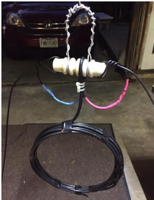
**Added weight from the choke coil (above) hung from the feedpoint and made from the coaxial transmission line. This choke prevents L3 antenna currents from flowing on the outside of the coax shield. This erroneous current can cause RFI and noise problems. It can also distort the radiation pattern of the antenna, but a low antenna at 3.9 MHz does not have a major radiation pattern distortion issue, as an HF Yagi would have, as it is already distorted into a ball shaped omni-direction pattern.**
