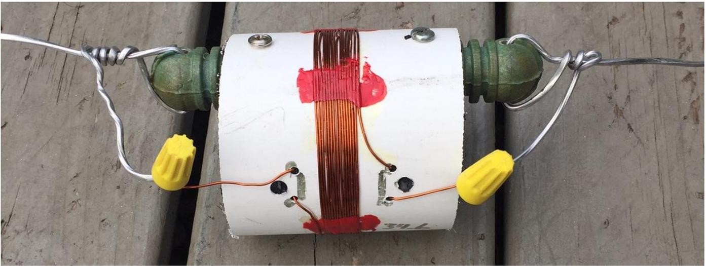
**Above prototype -- shows the attachment of the long insulators to the pvc coil form with self tapping machine screws. I did drill pilot holes for ease of installation. The wire nuts were used during testing in order to make the coil removal possible. I used #10 aluminum wire for the antenna wire because I had a lot of it, it was easy to bend and shape, it easily folds back on itself and shorts out.**
