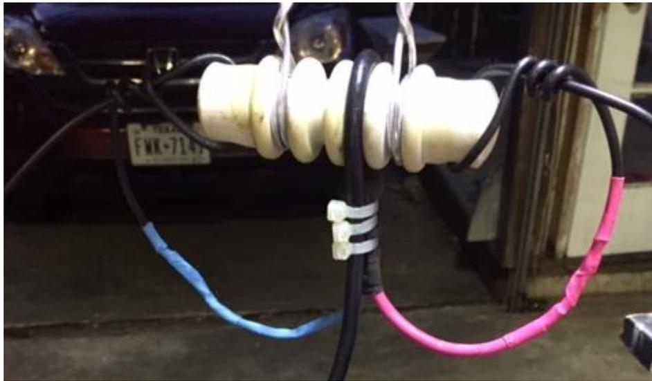
**The final center insulator connected to the antenna and coax**
